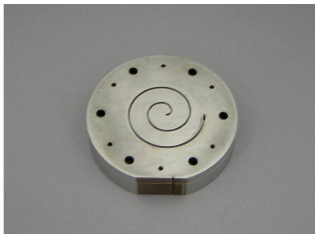
Fig. 5. Photograph of the microchannel plate used in reaction experiments (channel size = 0.8 mm (height) \times 1.0 mm (width) \times 113.0 mm (length), channel geometry = vortex).
